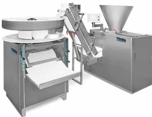
Round and long kneading machine combined with a Metra dough weigher, including a high conveyor.
